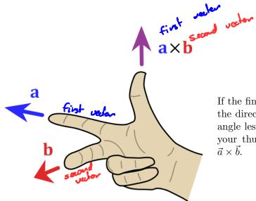
If the fingers of your right hand curl in the direction of a rotation (through an angle less than 180°) from  $\vec{a}$  to  $\vec{b}$ , then your thumb points in the direction of  $\vec{a} \times \vec{b}$ .
