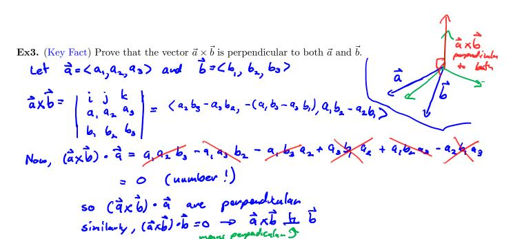
**Rmk:**  $\vec{a} \times \vec{b}$  points in the direction perpendicular to the plane through  $\vec{a}$  and  $\vec{b}$ .
